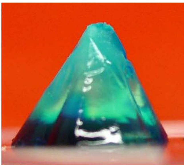
Figure 2 Hydrogel mold. Firm hydrogel formed in a conical mold. Green stain was applied to the bottom after complete gel formation, demonstrating diffusion into solid gel. Height of the sample is approximately 20 mm.
